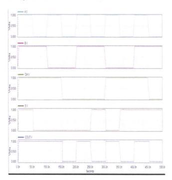
Figure 4: Simulation of Hybrid Full Adder17 T Transistor
