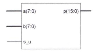
Fig.3.2: Block diagram of 8-bit booth multiplier
