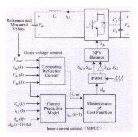
Fig. 5. The control block diagram for the UC.
