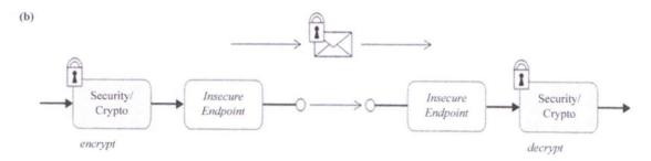
Figure 2. (a) and (b) Apache Camel Security Architecture [18]
