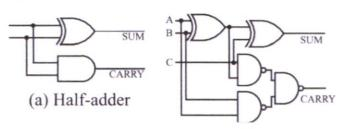
Figure 7. Half Adder and Full Adder
