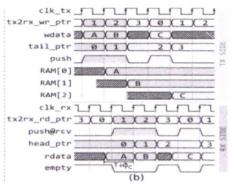
Figure 3. (a) Proposed mesochromous FIFO, which implicitly synchronizes data through the explicit synchronization of the flow-control push/pop signals. (b) Short cycle-by-cycle example of the operation of the proposed design.
