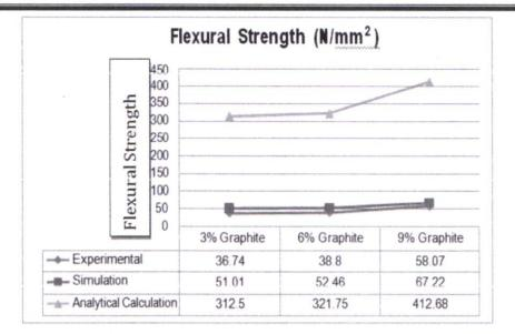
Graph 02: Comparison of Experimental, simulation and Mathematical relations (Flexural Test)
