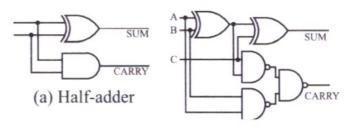
Figure 7. Half Adder and Full Adder
