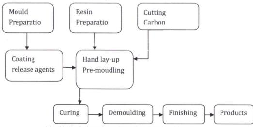
Fig. 03: Technique flow chart of FRP by hand lay-up
