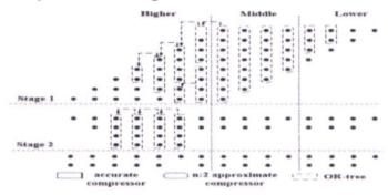
Fig.4.2:PPM Reduction In The Proposed Approximate Multiplier
