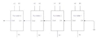
Figure 5. Ripple Carry Adder
