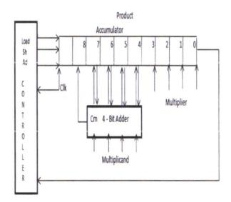
Figure 1: Multiplier Block Diagram
