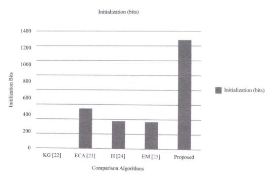
Figure 7. Communication overhead for Each Algorithm
