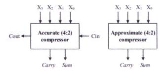
Fig. 4.1: (a) Accurate compressor
