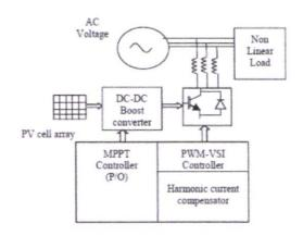
Fig. 3. Block diagram of PV- APF system
