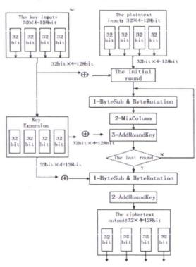
Figure 2. The new improved structure of AES algorithm
