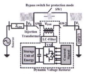
FIGURE 1. Basic circuit of power system with DVR.
