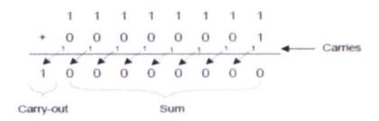
Figure 3: Binary Adder Example.
