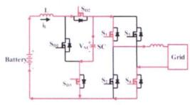
FIGURE 4. Flow path in active state of boost mode.
