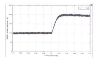
Fig. 2. The power response of the battery when the controller parameter  $\delta_i$  is changed.
