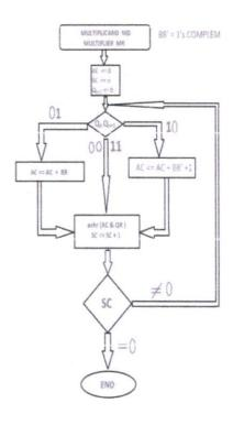
Figure 8: Booth's Algorithm Flowchart
