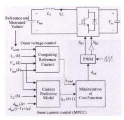
Fig. 4. The control block diagram for the battery
