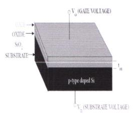
As shown in the figure, MOS structure contains three layers –
