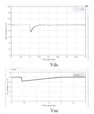
Fig. 1. System voltage response in the case of short-circuiting of the UC
