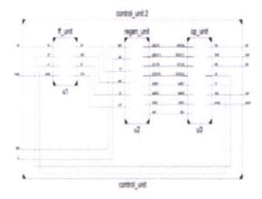
Figure 6 Block Diagram Of GCD Control Unit
