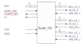
Figure 1:block diagram of four port router
