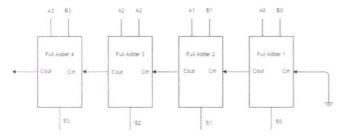
Figure 5. Ripple Carry Adder
