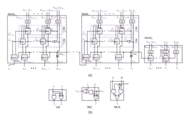
Figure 5: Multi-block carry select adder (a), and the gate-level designs of HA, INC and MUX (b).
