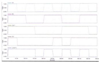
Figure 9: Simulation of Hybrid Full Adder-22 Transistor
