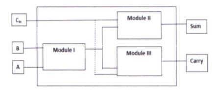
Figure 1: Block diagram of hybrid logic FA circuit
